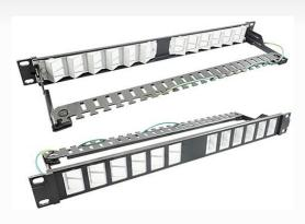
The flat 1U 24-port panel is design to accept keystone jack seated in angles inside the panel and result the connected patch cables automatically run to the cabinet/rack side to eliminate additional routing to horizontal cable manager/panel to save consumption of rack space. Flat design is ideal for installation within telecom cabinet as well as rack.
